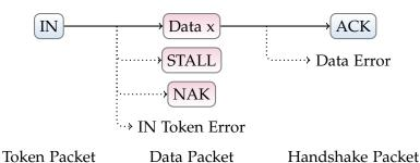
Again, it is possible that multiple data packets are needed, and the basic algorithm is the same as with host-to-device transactions. The relevant LUFA functions can be chained together, and will clear the IN endpoint bank after each full packet, but not after the last packet. The final packet has to be sent explicitly by calling Endpoint\_ClearIN().
