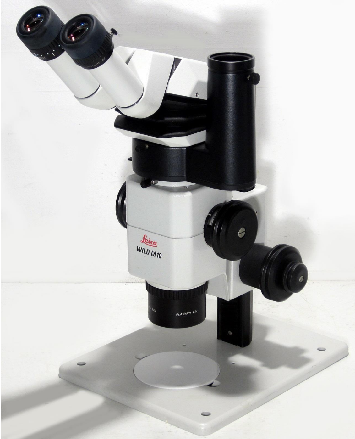
Figure 28. Wild M10 trinocular with planapo 1.0x CMO, Photograph courtesy and with permission of Sychrostream Solutions
