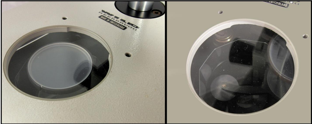
Figure 10. The Wild M3, results of using the rear lever to switch between bright field and dark field
