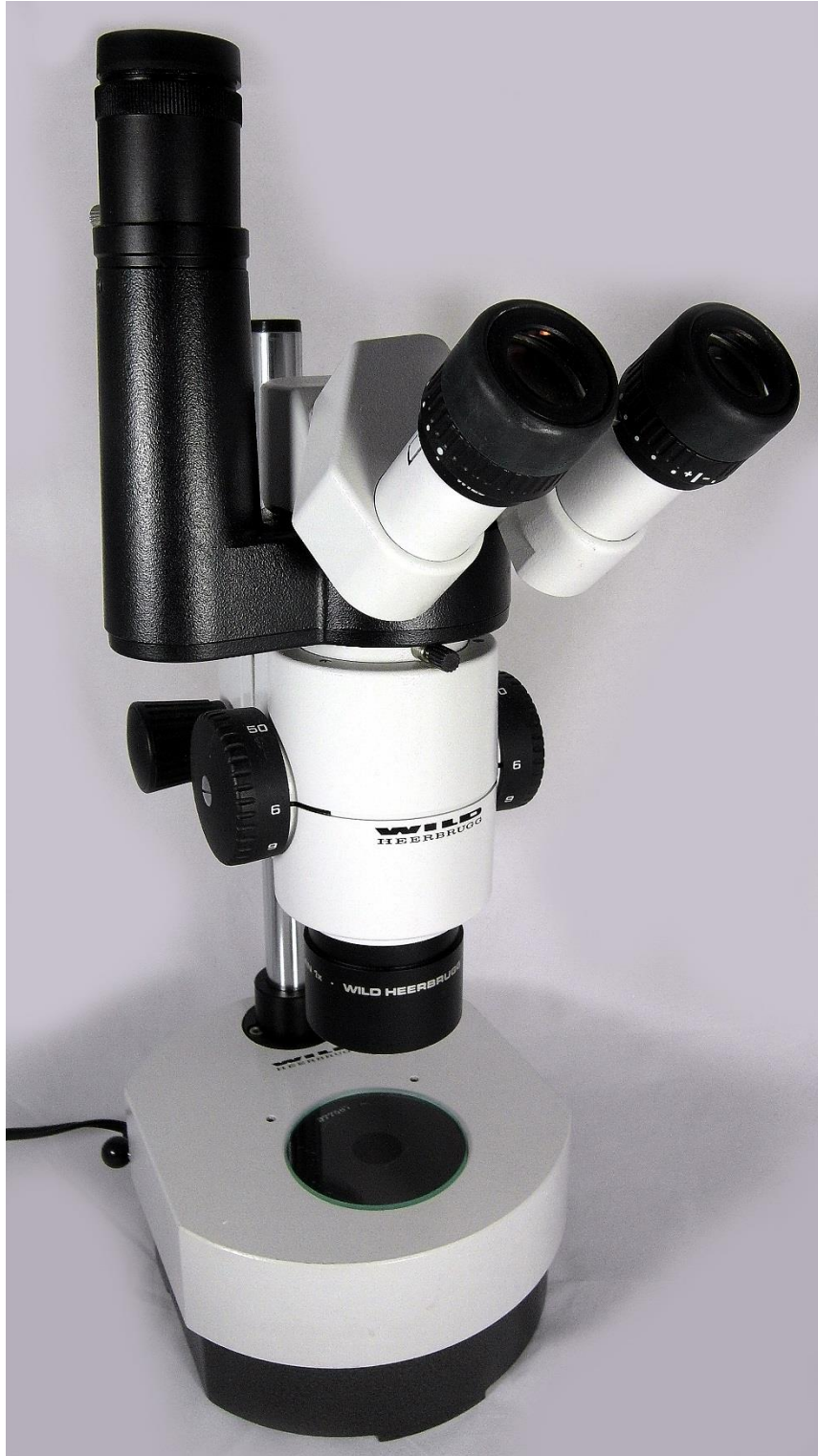
Figure 20. Wild M8 stereomicroscope with bright field/dark field transmitted-light stand
