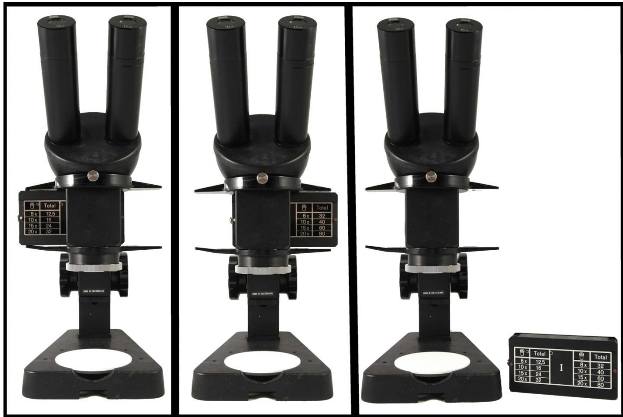
Figure 5. Wild M4 stereomicroscope, 1st style, showing three magnifications options
