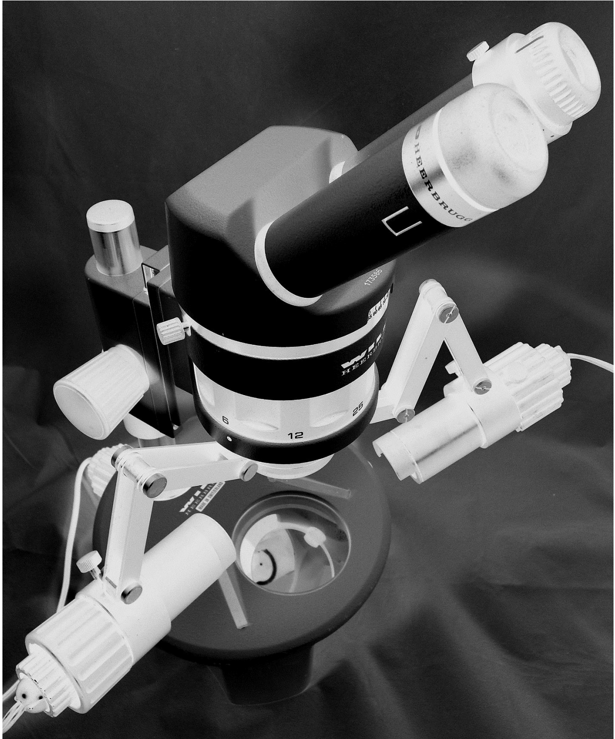
Figure 23. Wild stereomicroscope with triple illumination, two for incident and one for transmitted-light. Image inverted (white on black) to better show the lamps.
