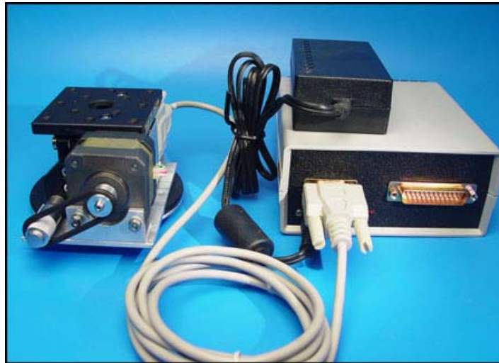
Figure 8. (left) Z-axis translation stage with stepper motor; (right) stepper motor driver electronics and 12-volt power supply (above).
