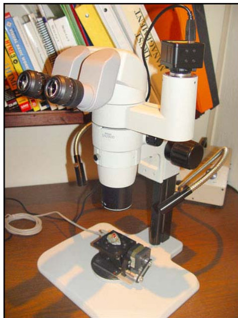
Figure 9. A research-grade Nikon SMZ800 trinocular microscope with digital camera and automated Z-axis stage.
