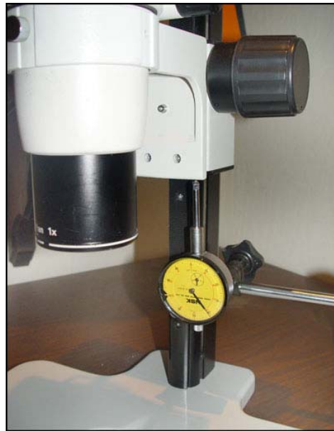
Figure 5. A machinist's dial gauge indicator that has been mounted on Nikon SMZ800 microscope to facilitate accurate measurement of the Z-axis position of the microscope head.
