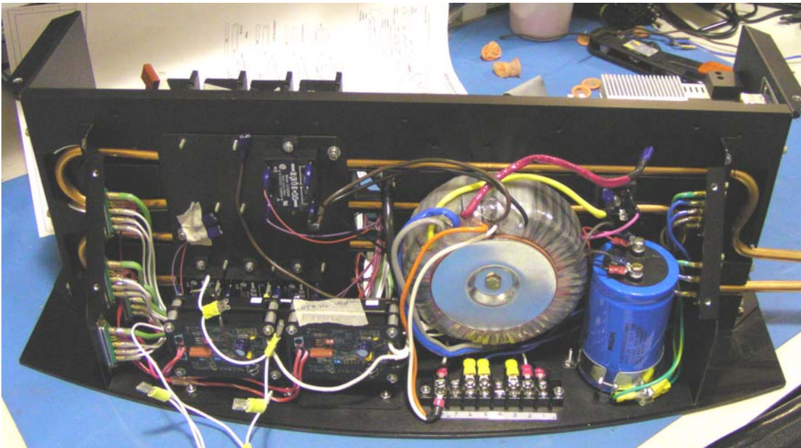
Figure 9. The reverse side of the electronics module containing the power supply for the servo amps and connectors. The optional cooling lines exit to the right.
