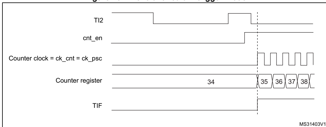
Figure 202. Control circuit in trigger mode
